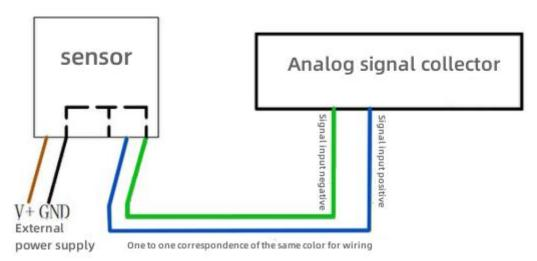
Example of connection method: schematic diagram of four-wire
